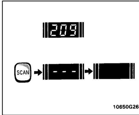
4. The three-digit code should be on the display. Push “SCAN”. The display will read “- - -”.
