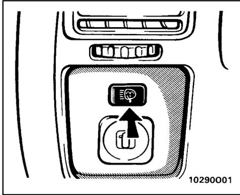
To spray fluid on the headlights, turn the headlights on and push the switch.
