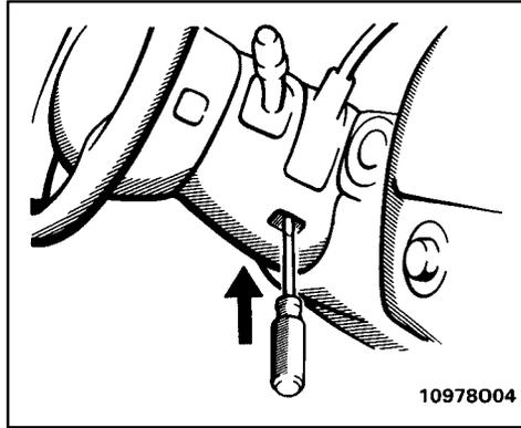
3. Insert the screwdriver or equivalent into the hole to push up the shift lock override button. You can shift out of “P” position only while pushing the button.
