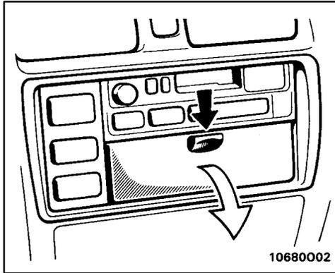
To open the miscellany box, press on the knob and pull out the box lid.
