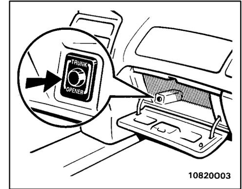
To open the trunk lid from the driver's seat, push the lock release button.
