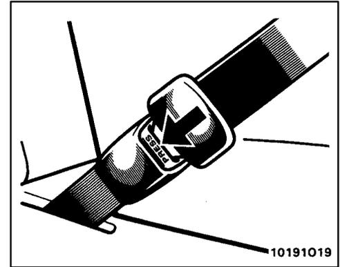
3. To remove the child restraint system, press the buckle-release button and unhook the top strap.
