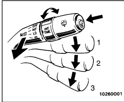
To turn on the windshield wipers, move the lever to the desired setting. The key must be in the “ON” position.
