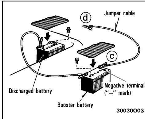
c. Connect the clamp of the negative (black) cable to the negative (-) terminal on the booster battery.
