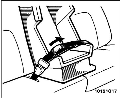
2. To hold the child restraint system securely, tighten the belt by pulling its free end while firmly pushing down the child restraint system.
