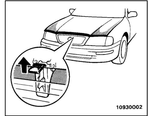
2. In front of the vehicle, pull up on the auxiliary catch lever and lift the hood. Before closing the hood, check to see that you have not forgotten any tools, rags, etc. Then lower the hood until make sure it locks into place. If necessary, press down gently on front edge to lock it.
