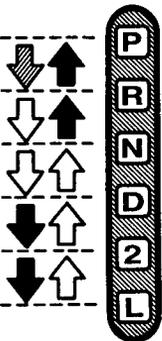
P — Parking, engine starting and key removal position
