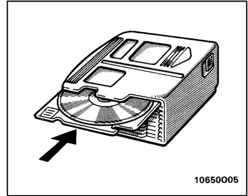
4. Place a disc on the tray with its label face up, and insert the tray into the slot. The magazine can store 12 discs of 12 cm (4.7 in.). The player will skip any empty disc slots.
